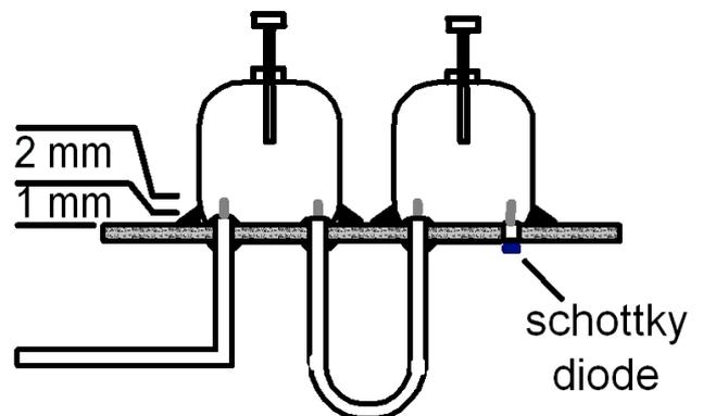
When fitting the U shape link, make sure both ends enter their respective board holes Perpendicular – the coax is slightly springy, and may have lost some of its shape.
