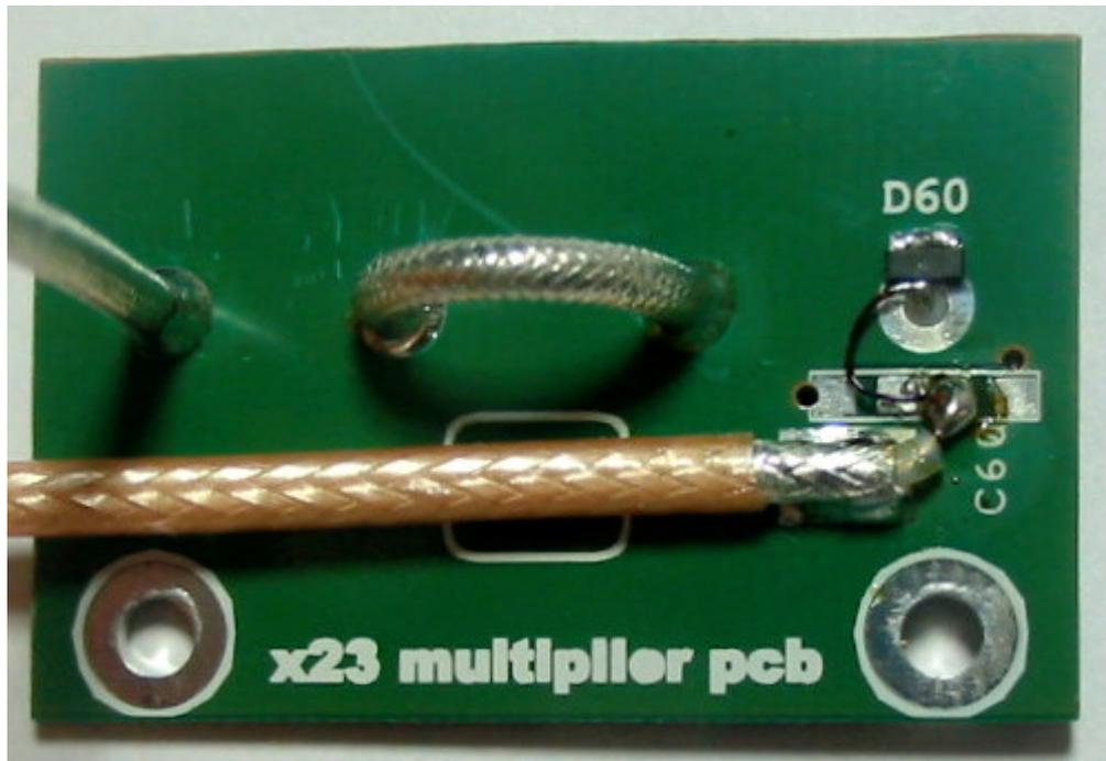
Both ends of the (RG316) coax lead have prepared ready for use. One end is cut back shorter than the other, and it is this end that should be soldered to the x23 multiplier board, as above. The inner is soldered to the junction of the C60/C61 pads (no capacitors are fitted).
