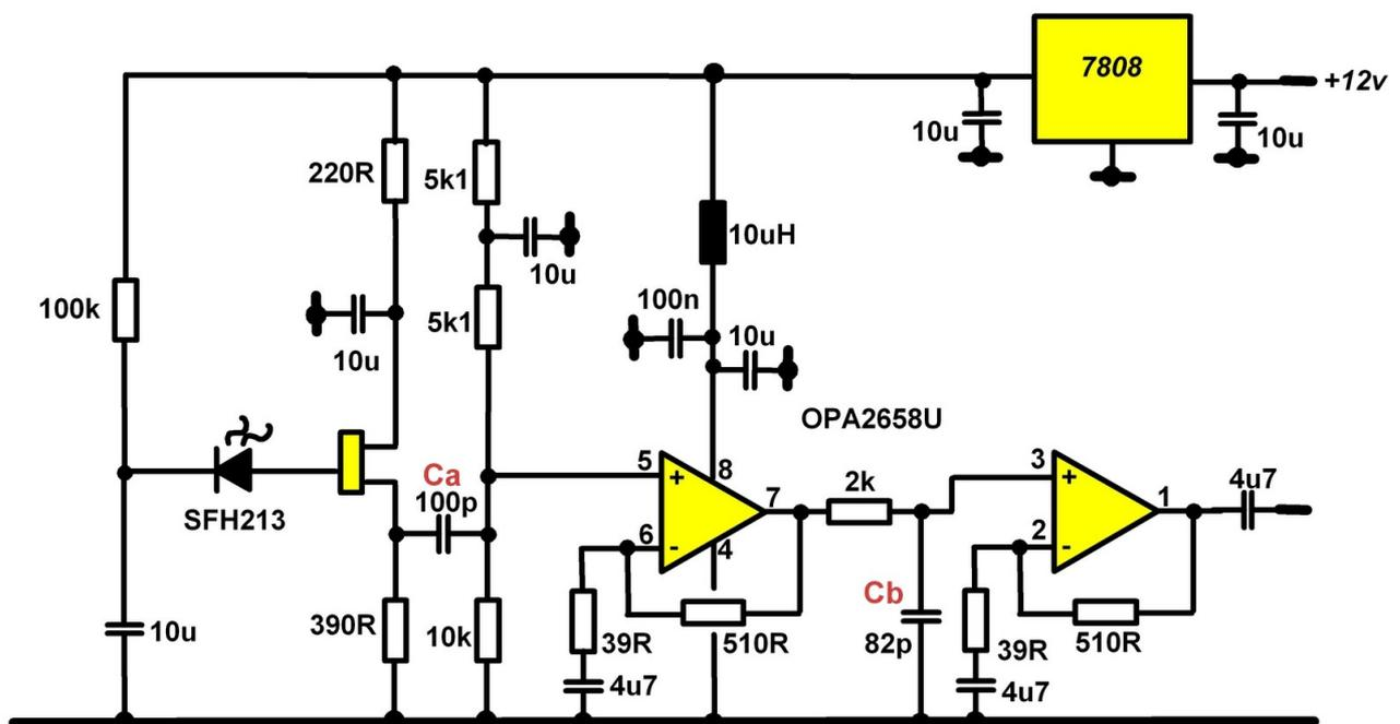
The OPA2658U op-amp maintains its gain well into the VHF spectrum, so to avoid any issues of amplified 2m noise making its way into the MiniTioune receiver, shunt capacitor Cb was added to the input of the 2<sup>nd</sup> op-amp stage.
