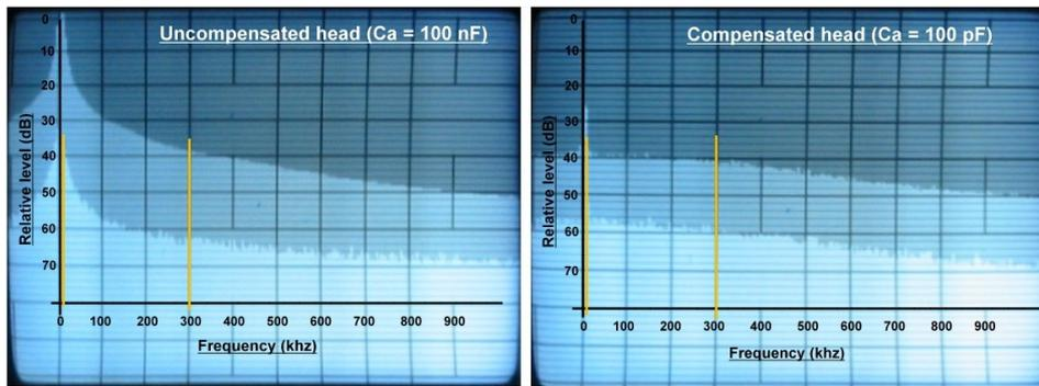
*Frequency response of optical head before and after frequency compensation
