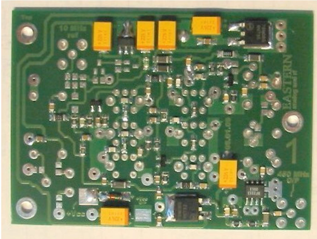
Board with RF2312 fitted at IC4
